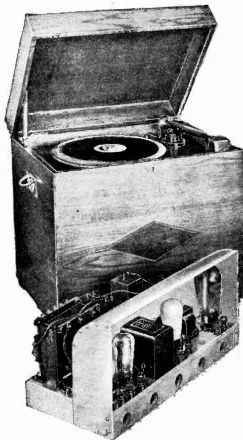
The amplifier shown separate from the cabinet. The synchronous electric motor, pick-up and the two controls are attached to the motor board.
