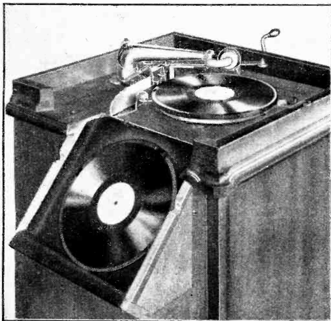
Produced at Hayes in 1920 and believed to be the first experimental automatic record changer. Five records could be handled.
