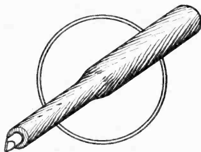
A simple form of insulated screwdriver, for adjusting trimming condensers. It is supplied with certain H.M.V. radio-gramophones.
