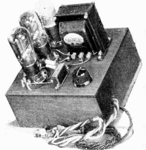
Three-quarter plan view of battery model. In the lower right-hand corner is the control knob of the grid bias potentiometer.
